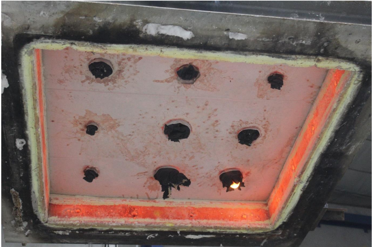
Figure 27 – Exposed face after the test
